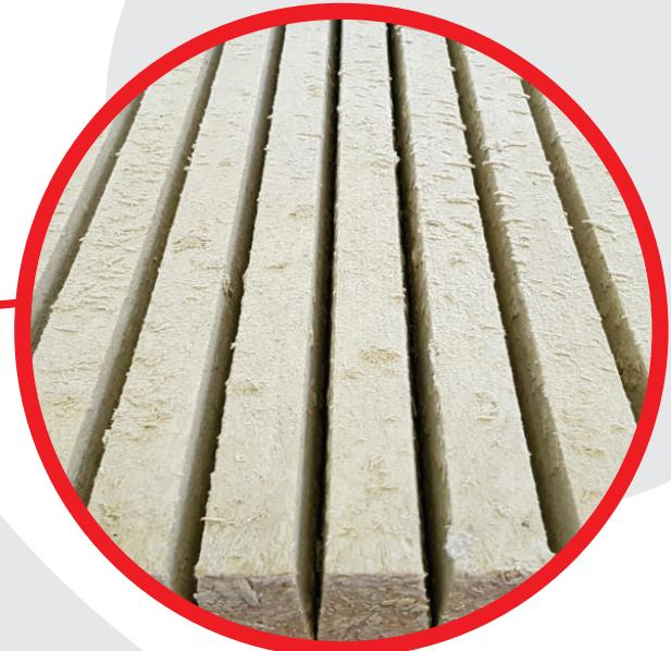
The insulation mats in the form of lamellas made of mineral wool with a high density, it is covered with reinforced aluminium foil. For the insulation of tank pipelines etc. They can be used as the first or subsequent layer of insulation.
